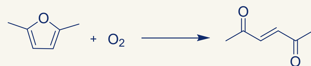
← The observed reaction of 2,5-dimethyl furan to form 3-hexene-2,5-dione
