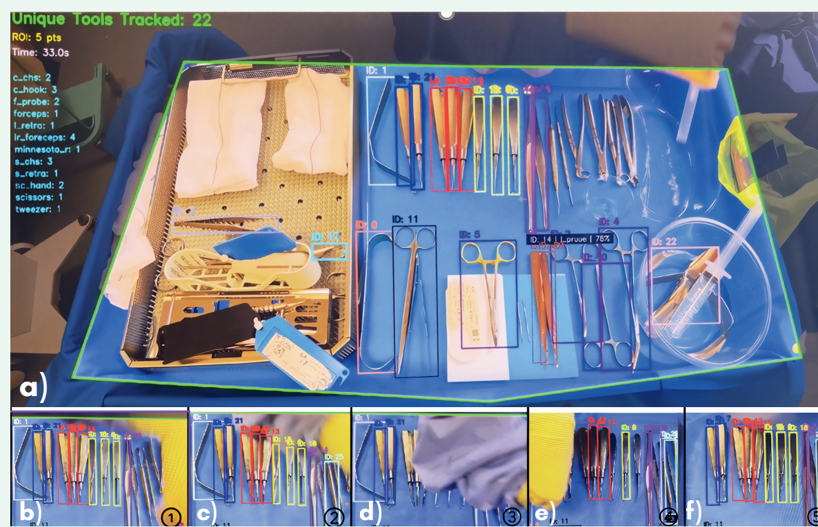
Figure 6. Tracking outputs: (a) ROI-constrained detections with instrument IDs; (b-f) sequential frames showing ID continuity across temporary occlusion.
