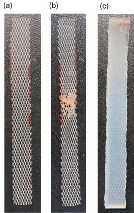
Figure 6. (a) PP mesh sample before testing. (b) PP mesh sample with tissue caught in the pores following testing. (c) Silicone-embedded PP mesh sample before testing.
