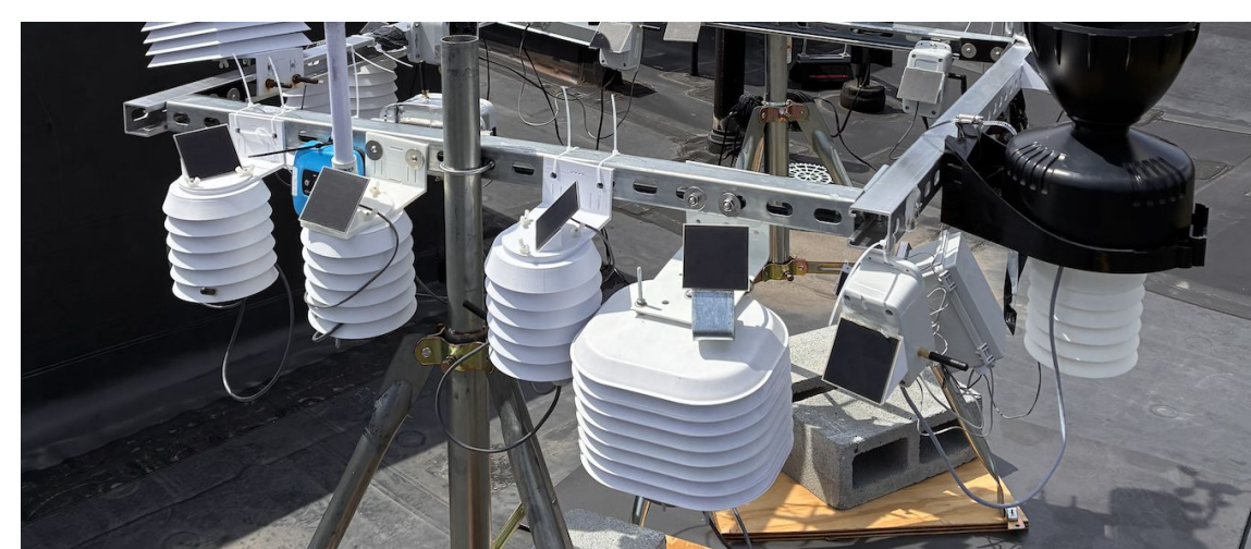
Above: Cross-sectional labelled view of the new assembly Right: Array of sensor set up on Lincoln Field; Three in-house shields and one Industry-made reference by Davis Instruments
